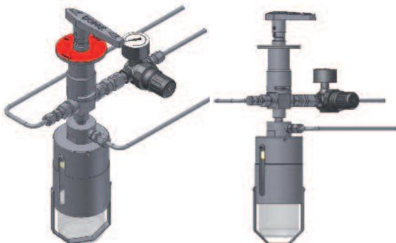
The ability to purge the needle assembly ensures there is no residue or build up in the needle assembly after retrieval of a representative, contamination free sample. The unit offers the possibility to purge the bottle with an inert gas prior taking a sample. The DPM type sampler in needle purge configuration allows purging through the needle assembly.
