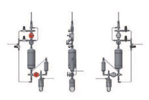
The ability to purge the sample point ensures optimal retrieval of a representative, contamination free sample. The S32 type sampler in overflow vacuum configuration provides a system purge to an overflow chamber and needle purge in addition to a fixed sample.
