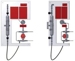
The ability to purge the sample point ensures optimal retrieval of a representative, contamination free sample. The S32-G type samplers provide a system purge to a flare connection in addition to sampling in a sample cylinder and the ability to depressurise the quick connect couplings before disconnecting the sample cylinder.
