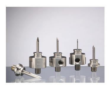
The needle assembly is the foundation of the DOPAK sampler for liquids. It is a housing with two integrated needles. The sample fluid enters through one needle (process) and displaced gas / vapour leaves through the other (vent).
