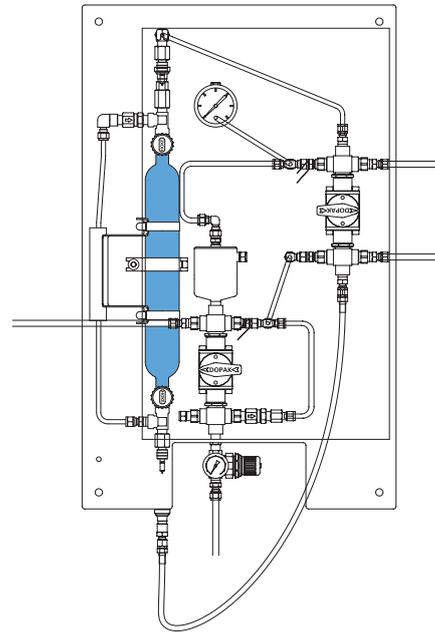
An extensive range sample cylinders are available, suited for sample collection, safe transport and chromatographic lab analysis. The sample cylinders are available in different volumes and material of construction. Cylinders are used for samples with high vapour phase, gas and liquefied gas. Standard sample cylinders are equipped with a needle valve on each side of the cylinder, a set of quick connect couplings and a carrying handle.
