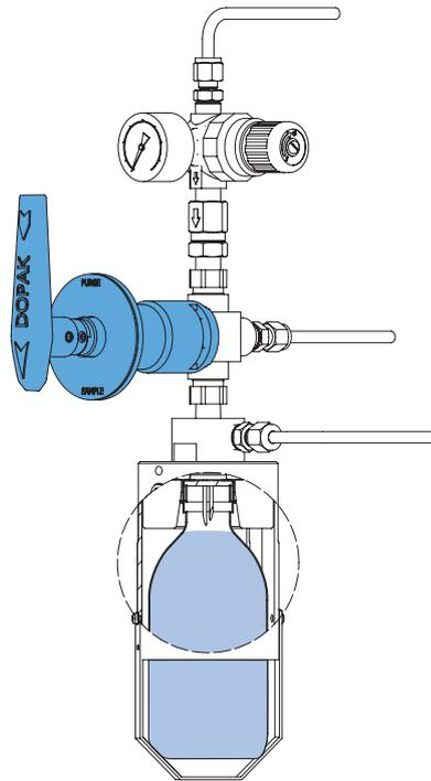
Different types of handles have been developed, serving the market's demand for more safety and ergonomics. Dopak spring return handles are suited for almost all valves used in Dopak sampling systems and significantly improve operator safety. When the handle is released, the sample valve returns to the "off" position.
