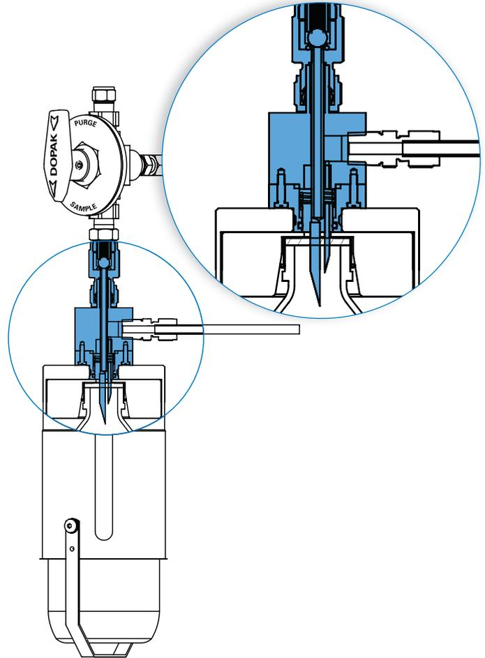
The unique design of the Dopak No Bottle No Flow (VTO-NBNF) is based on the conventional Dopak VTO needle assembly and includes a facility to prevent flow without a Dopak bottle with cap and a septum in place.
