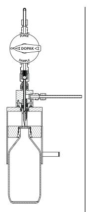
**0 - off**Without the sample bottle in place the VTO-NBNF is closed.
