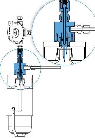
The unique design of the Dopak No Bottle No Flow (VTO-NBNF) is based on the conventional Dopak VTO needle assembly and includes a facility to prevent flow without a Dopak bottle with cap and a septum in place.
