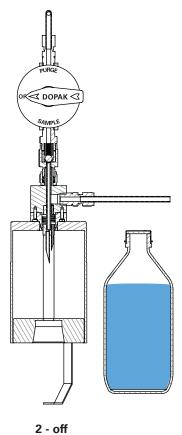
When the sample operation is finished, the bottle can be removed.
