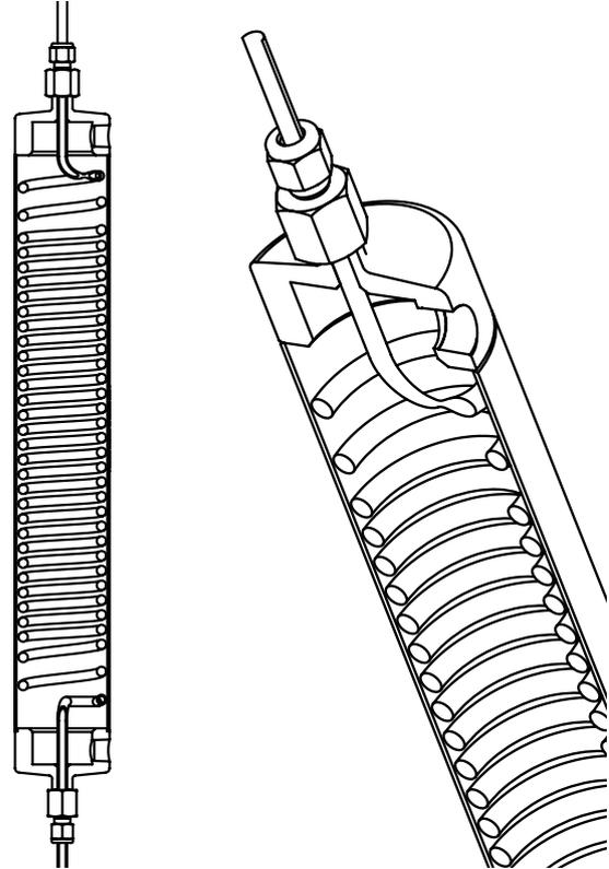
A Dopak single coil, tube/shell type sample cooler is an effective and efficient heat exchanger. The compact design makes it easy to install, next to a Dopak sampling system mounted on a stainless steel support plate. It protects the sampling system against high temperatures and ensures safe sampling.
