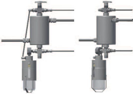
The ability to purge the sample point ensures optimal retrieval of a representative, contamination free sample. The S23 type sampler with cooling/heating jacket provides a system purge and a fixed sample volume at the required temperature.
